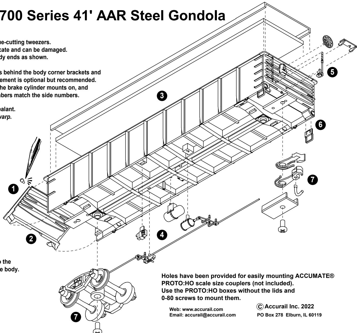
Holes have been provided for easily mounting ACCUMATE® PROTO:HO scale size couplers (not included). Use the PROTO:HO boxes without the lids and 0-80 screws to mount them.
